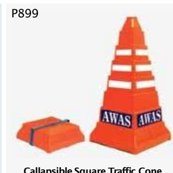
P899 Collapsible Square Traffic Cone Height 670mm Base size 300mm x 300mm Weight approx 2.5kg Material polyethylene medium density (PE)
